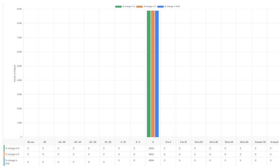
Figure 5: Impact (%) on N and P losses and GHG emissions resulting from the correction to ‘end crop’ event handling.
